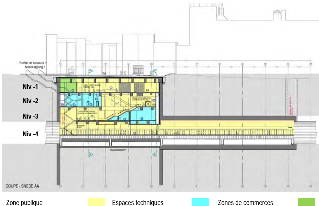
Figure 8 : Station Colignon, coupe longitudinale (BMN, 2018)
